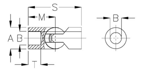
A = 36 B H7 = 18 M = 45.0 Max torque (Nm) = 120 s = 90 T = 22
